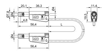
Highly flexible, with stackable  $\varnothing$  4 mm MULTILAM plugs with rigid insulating sleeve on both ends.
